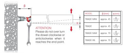
SCREW THE LOCKING BOLT TO BLOCK THE PIN
