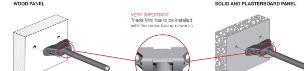
Recommended fixing pan head screw type - head Ø 5 mm max. It is the responsibility of the customer:
